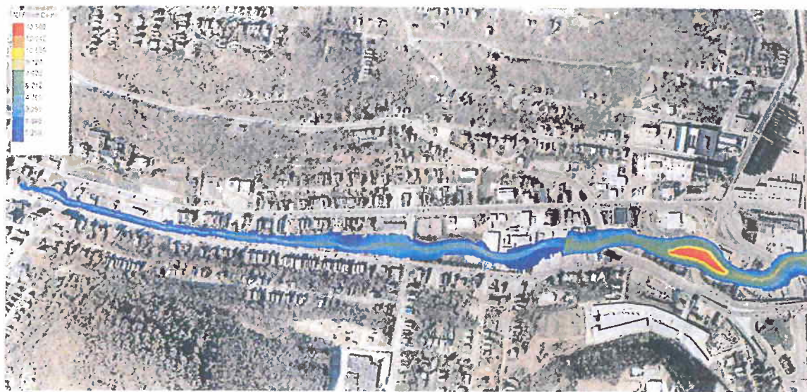
FIGURE 2- Projected Surface Flooding in the South Fairmount corridor during future conditions for 100 year storm event
